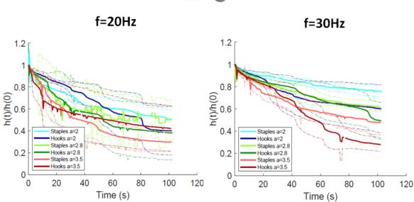
In general, as it was observed in the experiments, the staples appear to be more stable than the S hooks which is also shown in the right graph.
